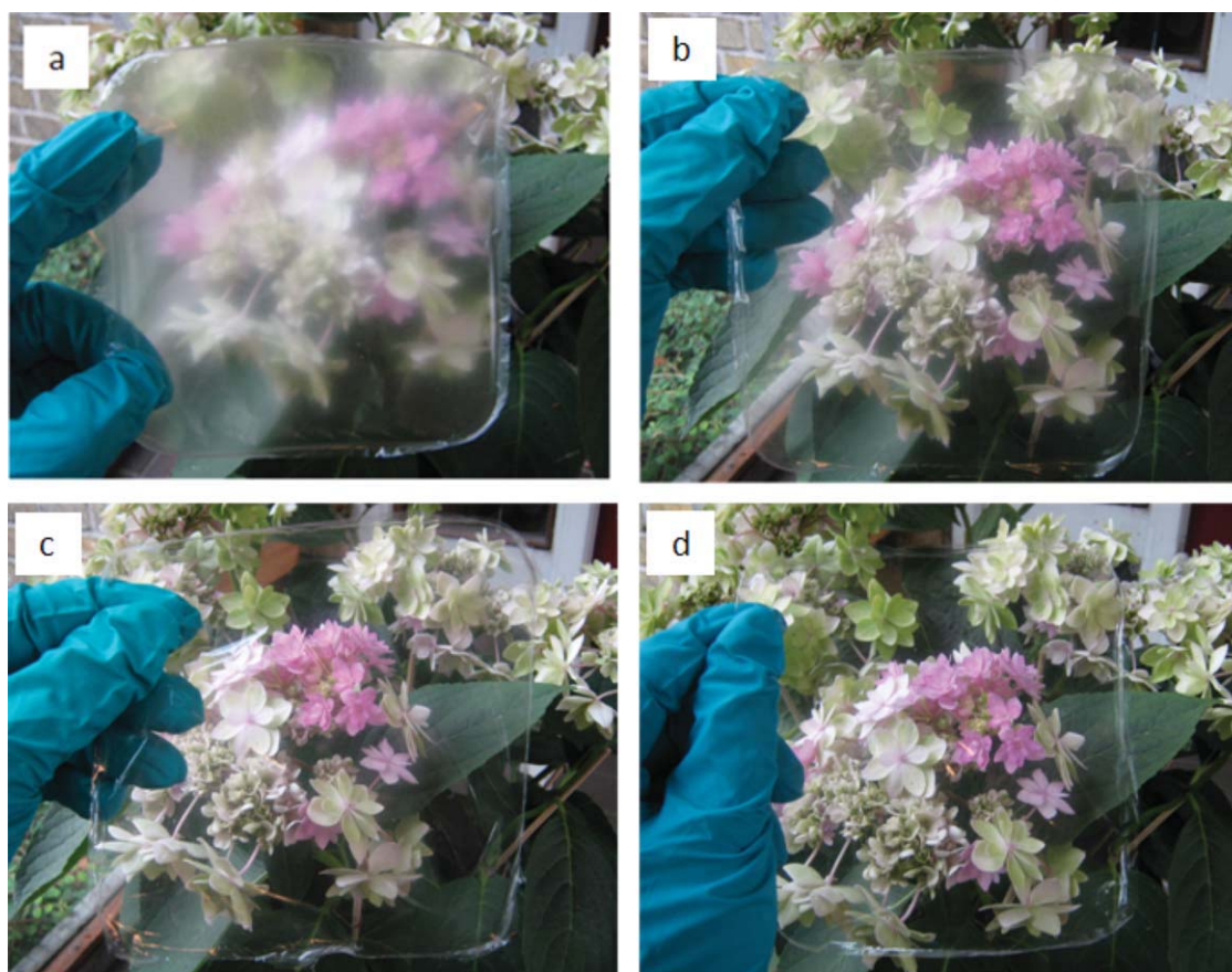
Figure 2 Visual transparency of the MFC 2 films: (a) 0p, (b) 1p, (c) 2p, and (d) 3p films. [Color figure can be viewed in the online issue, which is available at wileyonlinelibrary.com .]
